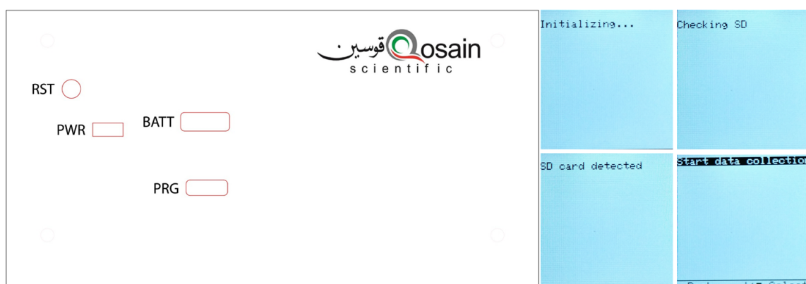
Figure 1: Left: Side view of the PM Tracker showing the BATT (USB-C) port, power switch, reset button, and PRG (programming) port. Right: Initialization stages of the PM Tracker.
