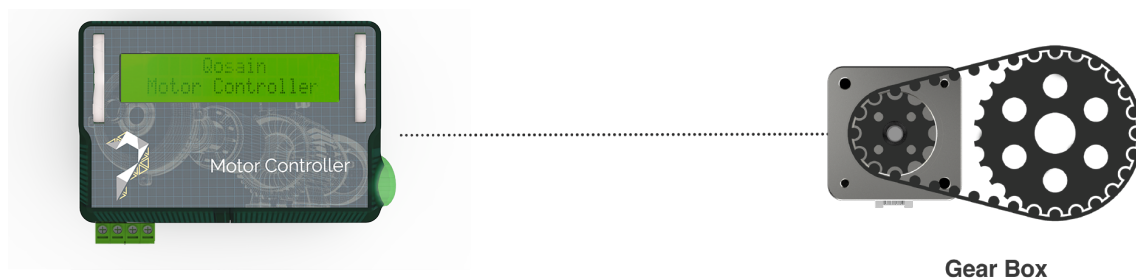
Figure 4.4: The hardware setup arrangement of the SMC when used with a gearbox (timing gears driven by a belt) mounted on the shaft of the motor.
