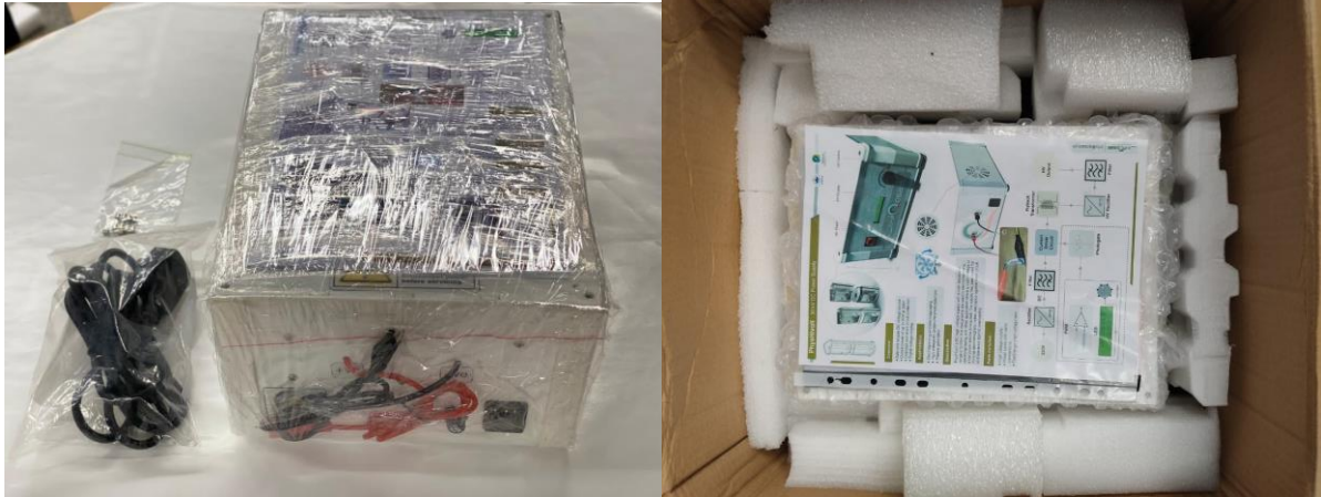
Figure 3 : The high voltage supply, after being adequately packed, needs to be placed in a cardboard box and supported by polystyrene sheets, before shipping.
