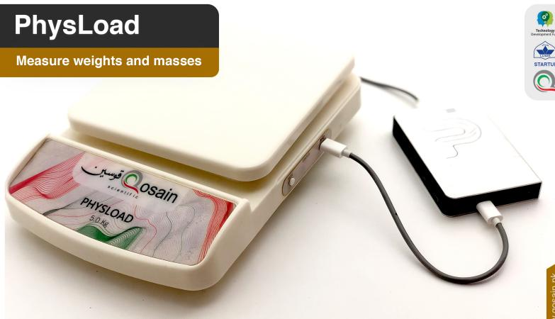
The **PhysLoad** is a modern, rugged and true to our spirit, low-cost balance that allows the measuring, recording, and plotting of mass in real time to offer an insightful demonstration of the dynamics of changing mass. The need of no prior configuration and inclusion of a hardware tare button (in addition to software control), make it an exceedingly simple instrument to operate.
